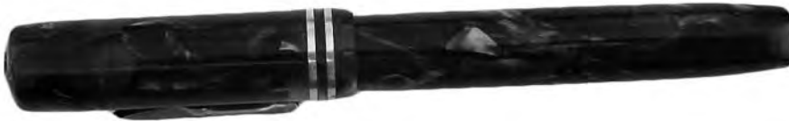
Conklin with crazing on both ends.
